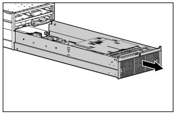
Figure 1-12: Removing the system board tray
